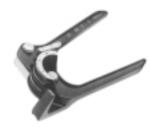
The 456 Tri-Bender is designed to easily bend there different sizes of soft tubing: 1/4", 5/16" and 3/8" with the same tool. Ideal for plumbing and HVAC applications. A 90° start angle minimizes effort required to form a bend. Handy reference marks indicate the angle for quick bends through 90°.
