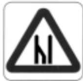
[13] CENTRE LANE CLOSED
