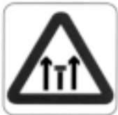
[17] CENTRE LANE CLOSED
